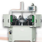
WJ-HD102 雙層鋁輪圈鑽孔機 Double-Walled Alloy Rim Spoke Hole Drilling Machine
